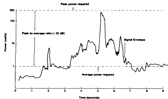
All loudspeakers are capable of sustaining short peaks of power *much higher than they can sustain on a steady, continuous basis*, and the proper choice of amplifier is quite dependent on the loudspeaker's ability to do this.
