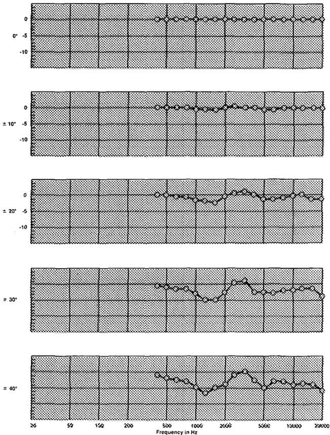
**Figure 4.** Vertical Off-axis Response (normalized):
