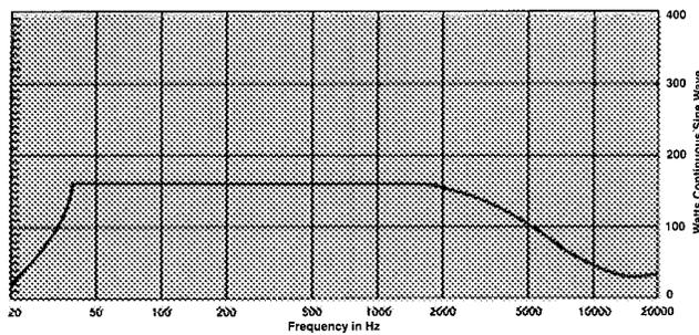
Figure 10. Maximum Continuous Output
