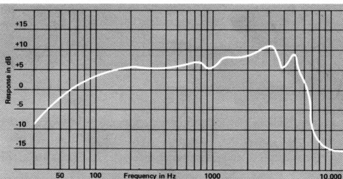
Frequency response contour of the 2120 in a closed box of six cubic feet internal volume. Measured response of a typical production unit, including all peaks and dips, does not deviate more than 2 dB from the above curve. Additional acoustic loading (a port) will further extend bass response.
