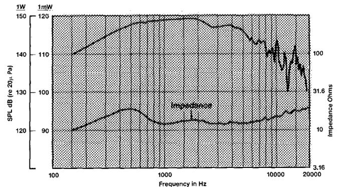
Frequency response and impedance modulus of Model 2450J coupled to a 49 mm (2 in) diameter terminated plane-wave tube, with sensitivity referenced to a 25 mm (1 in) tube. This is the power response of the transducer, and is the frequency response that will be obtained on a true full-range constant directivity horn design, such as JBL's 2360 series of Constant Coverage Bi-Radial® Horns.
