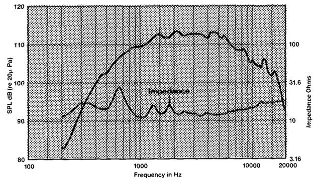
Frequency response of the 2450J coupled to a JBL 2380A Flat-Front Bi-Radial® Horn, measured on-axis at a distance of 1 meter with a 1-watt (4.0 V RMS) input in a reflection-free environment, with impedance vs. frequency curve. A horn with a pure exponential flare, such as typical radial horn designs, will exhibit greater high frequency output on axis at the expense of lost annular coverage.
