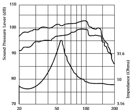
The pink noise signal was low-passed 100 Hz, with no electrical boost at low frequencies. Note that, for two different averaging setups, the response from 25 to 80 Hz remains flat over a very narrow range.
