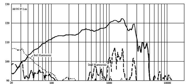
In comparing the curves on the 2241 H and 2242H shown in Figure 3, we must carefully take into account that the distortion of the 2241 H has been raised 20 dB, while the distortion of the 2242H has been raised 30 dB. This, in essence, makes the distortion of the 2242H look 10 dB greater than it really is, compared to the 2241 H. At 80 watts input, the third harmonic distortion of the 2242H is about 10 dB lower at 40 Hz than that of the 2241 H, while second harmonic distortion is about the same.
