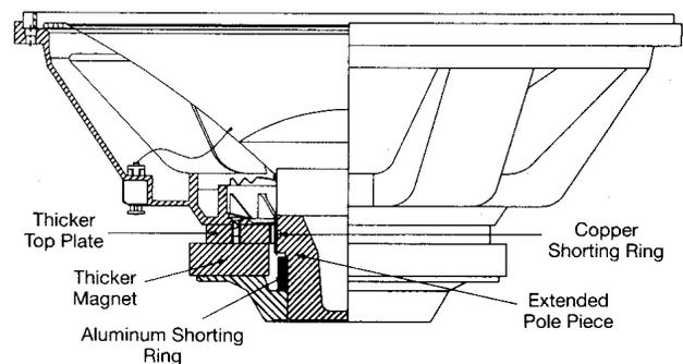
2. Extended pole piece. The extension of the pole piece above and below the gap provides better axial magnetic flux field symmetry for lower distortion at high excursions. At the same time, it provides better thermal conductivity for heat generated in the voice coil because of its proximity to the coil at all positions of its excursion.
