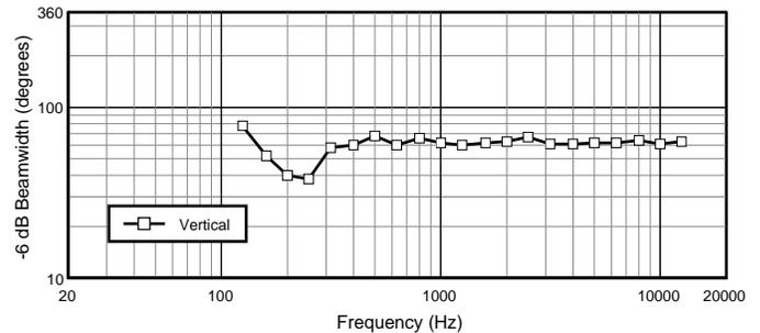
**Vertical Beamwidth, Six Element Array
