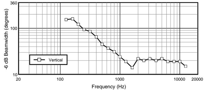
**Vertical Beamwidth, Two Element Array
