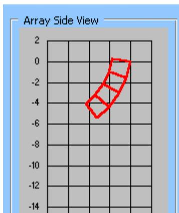
Figure 7. : Side view of 4-box VT4889 Array, 10-degree splay angles between baffles
