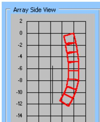
Figure #10. : Side View of 8-Box VT4889 Array, configured as a progressive line array
