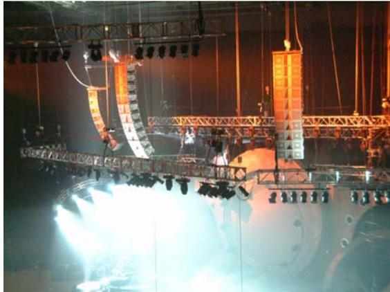
Figure #13. : VT4889 triple-array setup for asymmetrical seating area in multi-purpose sports arena.
