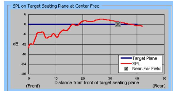
Figure #15. : Predicted SPL on main floor seating plane at 2k Hz center frequency, in venue with very high suspended arrays.
