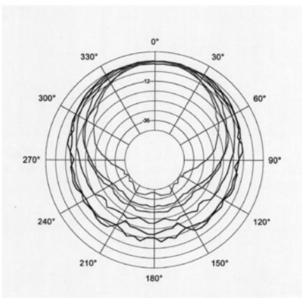
Figure 5. : Horizontal polar response of a single JBL VT4889 modular line array element.
