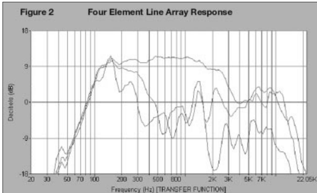
Here is the on-axis, 45° off-axis, and 90° off-axis response of a four element line array. The on-axis level goes up by +12 dB relative to a single element, and the
