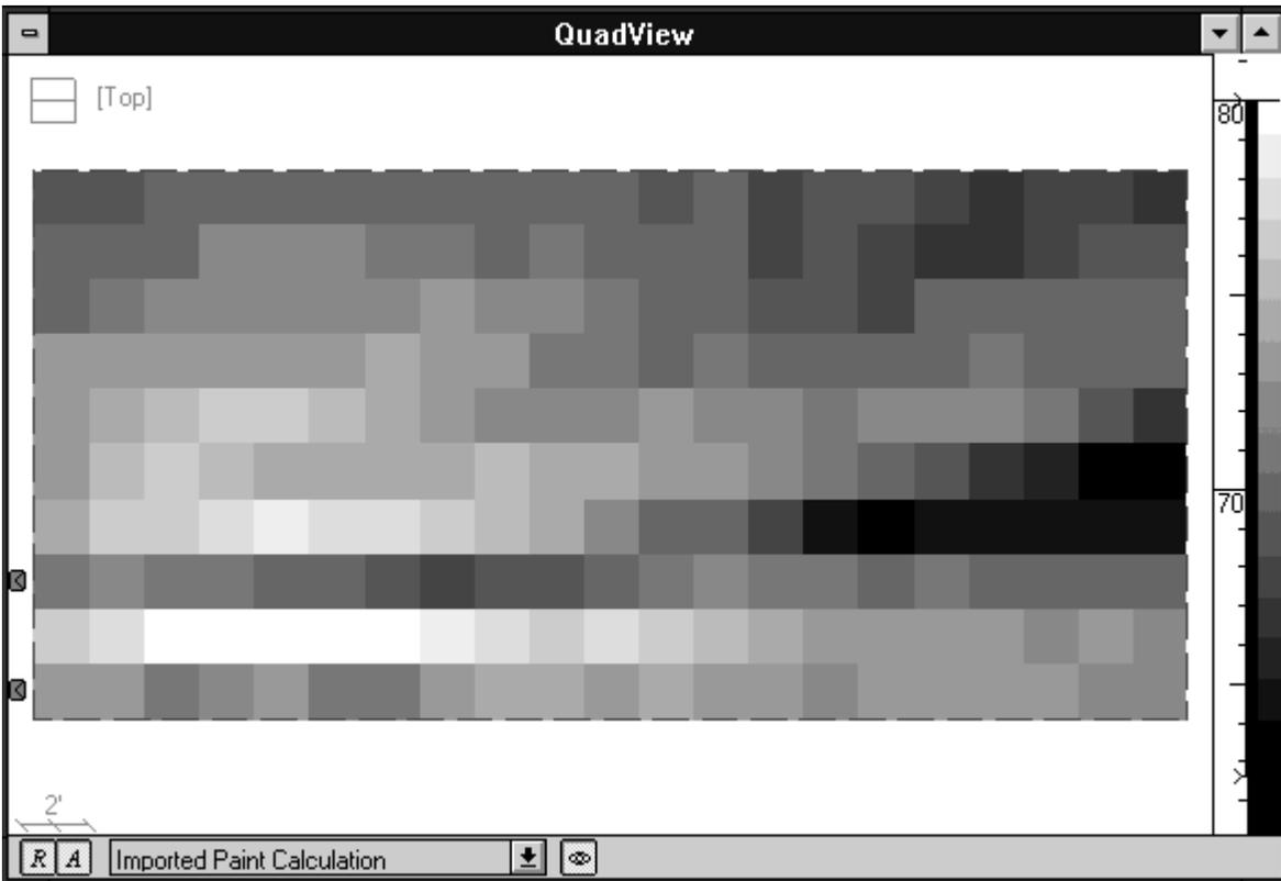
**Figure 4. Measured SPL for 2 sources @ 4' separation (2' resolution, uncalibrated)**
