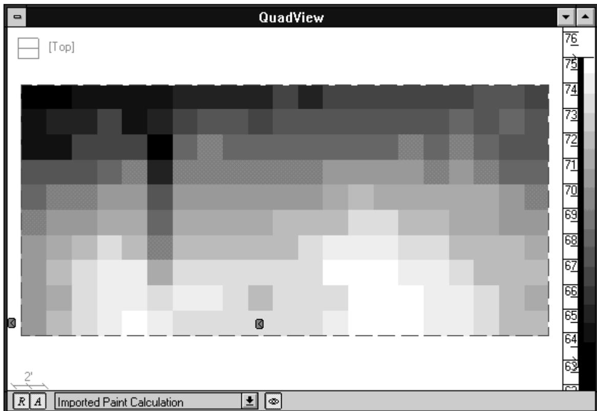
**Figure 8. Measured SPL for 2 sources @ 20' separation (2' resolution, uncalibrated)**
