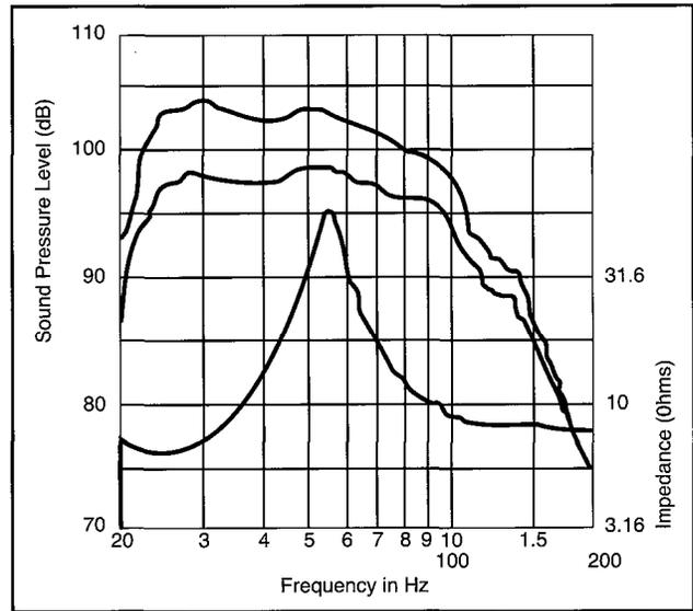
4645B frequency response, 1 watt at 1 meter, with equalization, 1 π (top curve) and 2 π (center curve) conditions.
