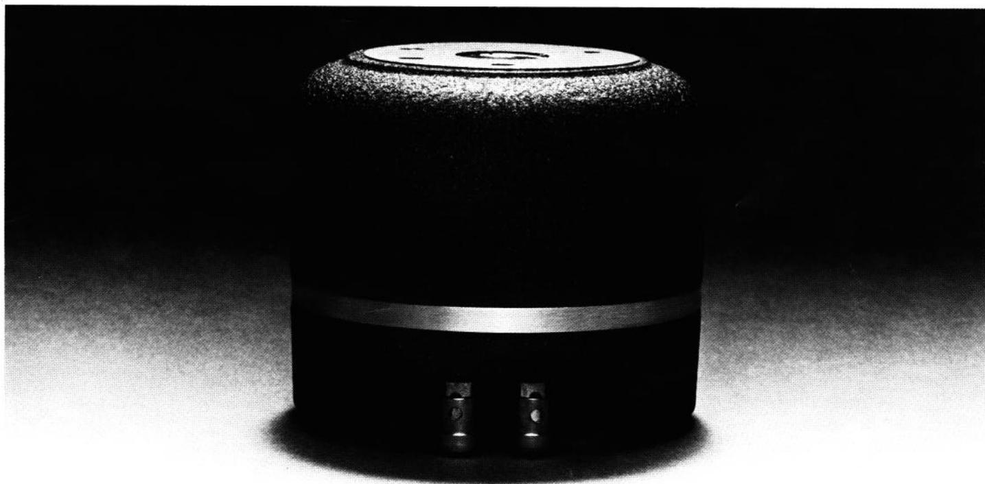
Model 2461 is an exceptionally rugged professional quality compression driver. Despite its small size, it has high power handling capacity and extremely high sensitivity, making it ideal for sound reinforcement systems where space is at a premium but sound quality cannot be compromised. The 2461 incorporates a phenolic-impregnated linen diaphragm, a concentric exponential phasing plug, 44-mm
