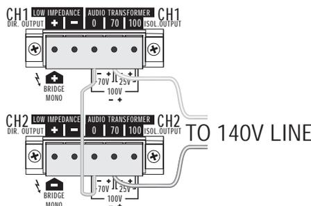
Output connections for “T” models, bridged mono mode, 200 volt line
