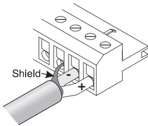
**Balanced Connection**—Attach as shown. Connect the (+) wire, (-) wire and ground wire to terminal pins as marked.
