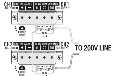
When operating the amplifier in bridged mono mode, neither of the speaker wires is at ground potential. Grounding either of the speaker wires can short out one side of the power amplifier. Use the same precautions in handling and dressing the wire as you would for the normal “hot” outputs. Ensure that neither wire connects to ground anywhere along its length. Do not use grounded autoformers on the loudspeakers.
