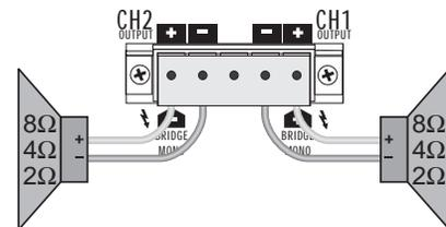
Output connection for MPC “T” models, bridged mono mode.
