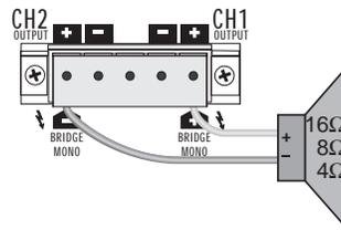
Output connection for MPC, parallel or stereo mode.
