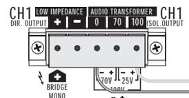
Output connections for “T” models, bridged mono mode, 140 volt line
