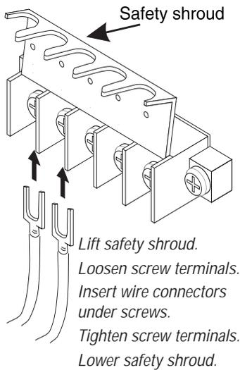
Covered barrier strips located on the rear panel allow safe, shockproof speaker cable connections to the amplifier outputs. See the diagrams for details on connecting speakers and/or distributed (25V, 70V, 100, 140V, and 200V) lines. Insulated connectors of the type shown are recommended. Always make sure the amplifier is turned off before you change any output connections or before lifting the safety shroud.
