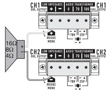
*Audio transformer*—For bridged mono operation using the *AUDIO TRANSFORMER* outputs, a jumper wire *must* be connected between the *AUDIO TRANSFORMER* “0V” terminals of the two channels. See hookup diagrams.
