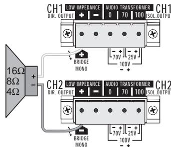
Output connection for MPC “T” models, direct low impedance.
