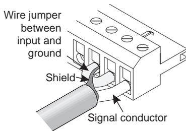
**Unbalanced Connection**—Attach input signal wires as shown. Use the non-inverting (+) input and the ground terminals of the header, and also connect a wire jumper between the inverting (-) input and the ground terminal. The wire jumper will prevent a reduction in gain caused by a floating unbalanced input.
