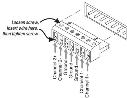
MPC amplifiers feature balanced inputs, connected via a Euro-style 7-terminal detachable header.
