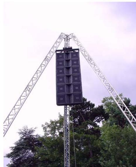
JBL VERTEC Array, weighing only .435 metric ton (960 lbs.), high atop SSE Hire's proprietary Teepee ground support system.
