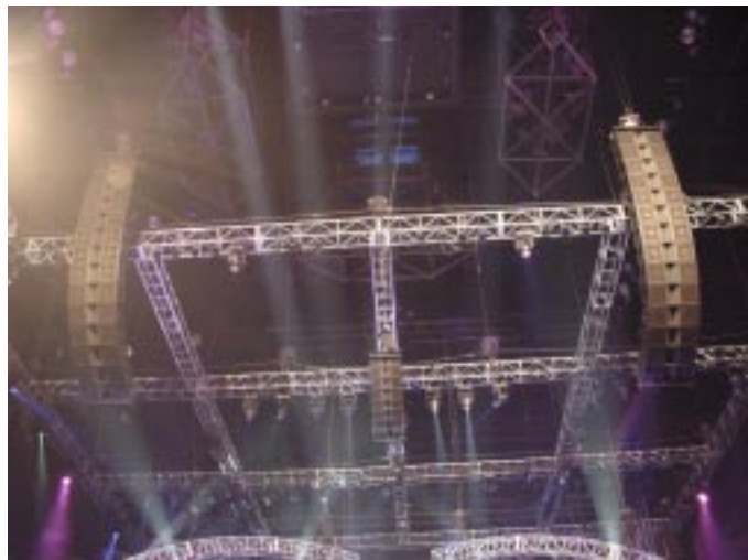
Florida's Acotech provided JBL VerTec VT4889 line array elements with compact VT4887s and VT4880 subwoofers for the 2003 Billboard Latin Music Awards at Miami Arena.
