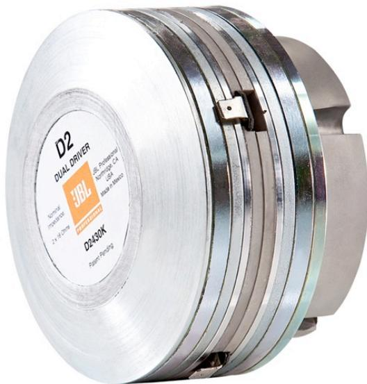
“With two smaller diaphragms and voice coils working on the same acoustical load, the VTX Line Array Series provides high efficiency and SPL, plus increased extreme high-frequency reproduction due to the smaller moving mass of each diaphragm and voice coil,” said Paul Bauman, Senior Manager, Tour Sound, JBL Professional. “The D2 Dual Driver is a radical departure from traditional compression drivers and represents a monumental breakthrough in loudspeaker system design!”
