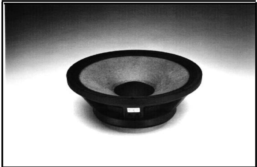
The 2227H is intended for use in applications where large amounts of low distortion wide-band acoustical power is required, along with excellent mid-bass transient behavior. It is ideal for such applications as stage monitoring systems, with their typical small enclosures, and as a driver for bass and mid-bass horns. The total peak-to-peak excursion of the moving system is 10 mm, within 10% linearity. JBL does not recommend the use of the 2227H transducer in subwoofer systems.
