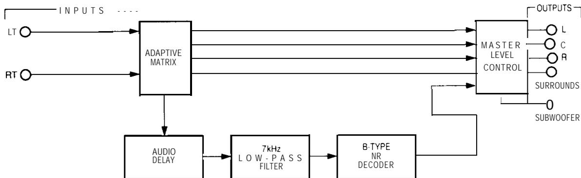
Figure 2B. Block diagram of the Dolby Stereo Optical playback matrix
