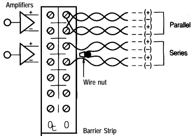
Figure 32B. Wiring at barrier strip in the booth
