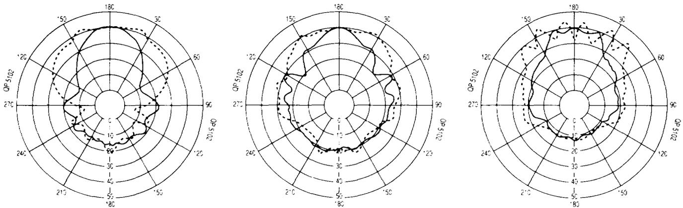
Multicellular horn (2 x 5) 1000 Hz vertical (so/id); horizontal (dashed)
