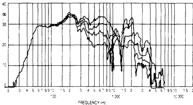
C. Reverberant (power) response of a cinema system composed of elements similar to those shown in Figures 5A and 5B
