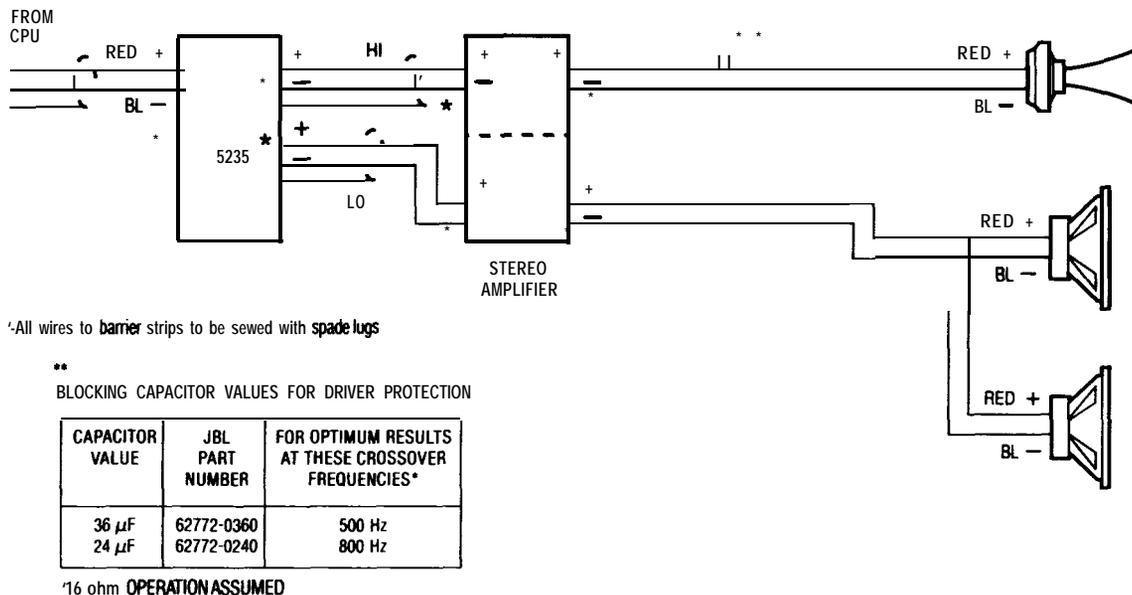
Figure 29. Wiring diagram for a bi-amp/i&d system
