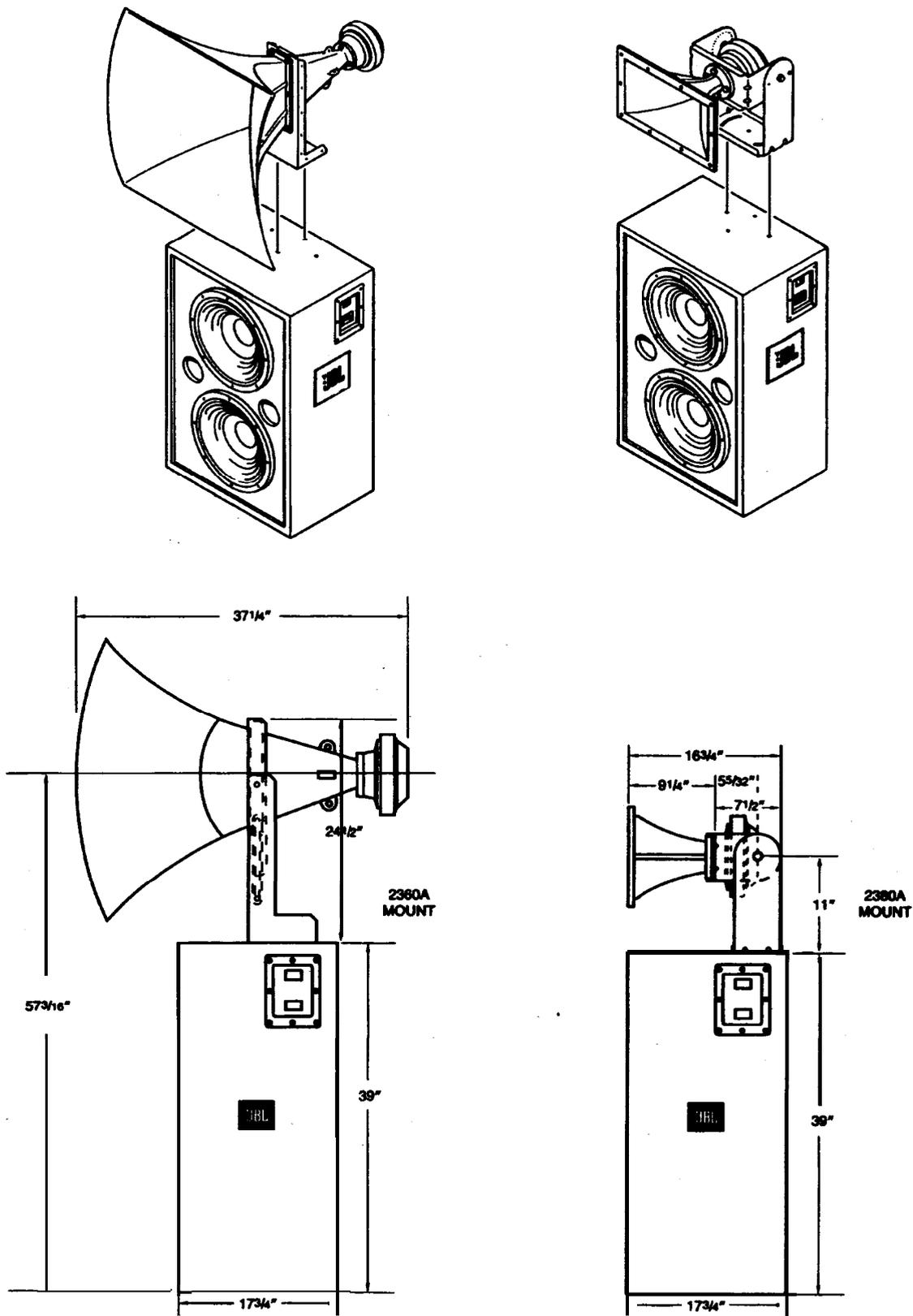
Figure 14. Complete system assembly diagram for 46700 and 46756.
