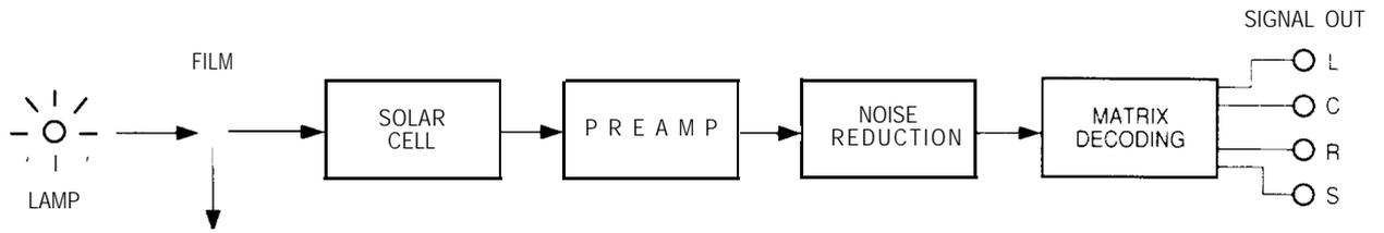
Figure 4A. Block diagram of analog A-chain
