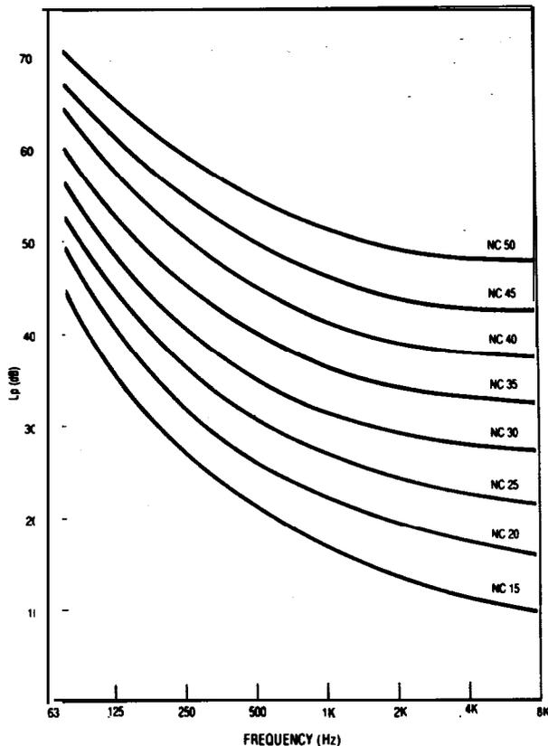
Figure 9. Noise Criterion (NC) curves, octave band data
