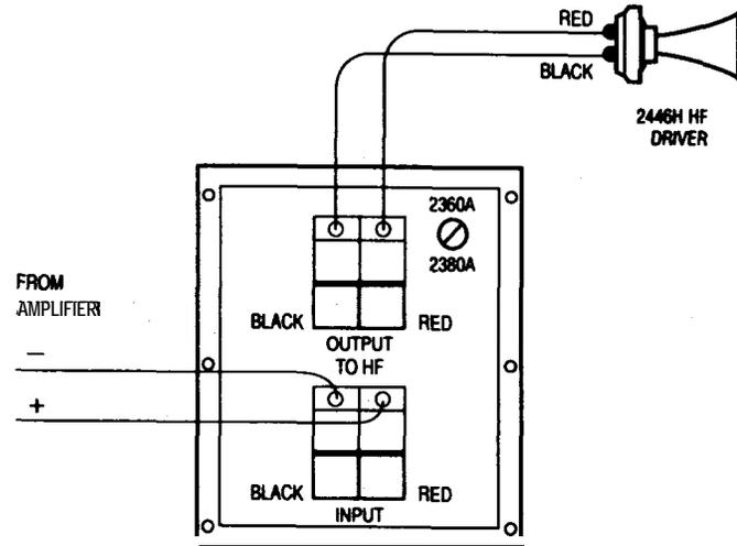
4675C wiring diagram
