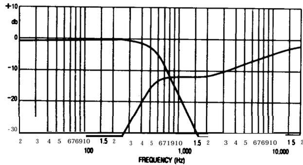
B. 500 Hz 18 dB/octave, with power response correction for 2360A Series horns
