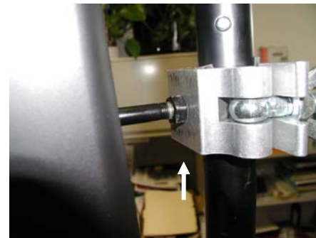
STEP 4 – Make sure that the nut on the Invisiball shaft is very tight to the cheeseboro clamp (just to make sure the speaker doesn't accidentally rotate).
