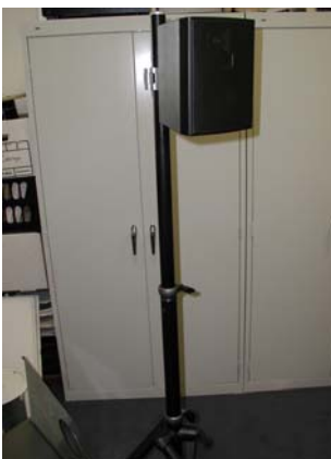
STEP 5 -- Adjust the aiming angle of the speaker using the Invisiball mechanism via a hex wrench from the front of the speaker and raise the stand.
