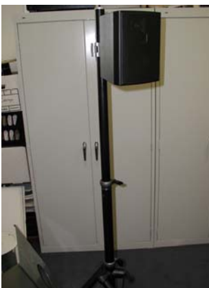
STEP 5 -- Adjust the aiming angle of the speaker using the Invisiball mechanism via a hex wrench from the front of the speaker and raise the stand.
