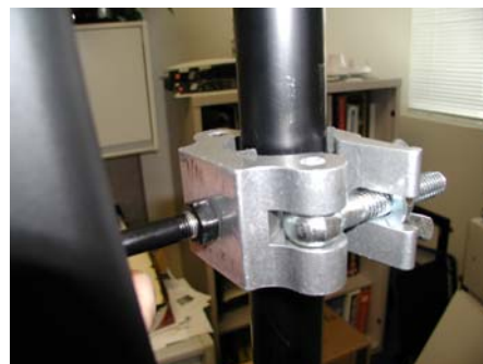
STEP 2 – With the wingnut loosened, place the clamp on the speaker stand. Flip the bolt into place (as shown).
