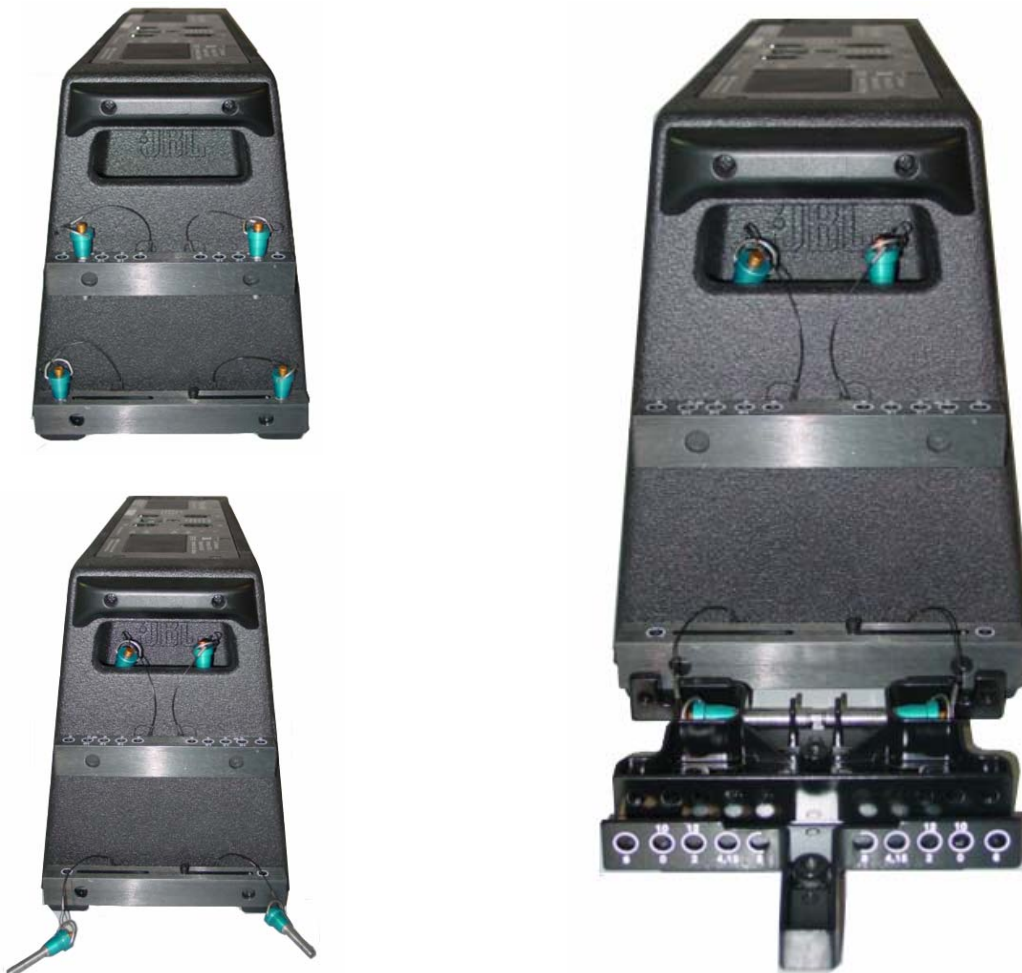
Figure 8: Left/Right Speaker Attachment Adapter Plates secure to VT4886 enclosure sides using supplied ball-lock pins. For suspended configurations or fixed installation, use #1/4-20 x 2" allen bolts and lock nuts for front attachment.
