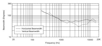
Measurements obtained in bi-amplified crossover mode
